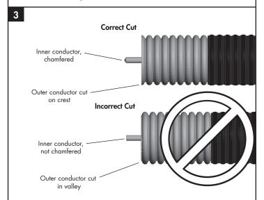
Check the cable to be sure that the outer conductor is cut at the top of a crest, that all cuts are clean, that the inner conductor is chamfered, and there is no debris on the surfaces.
