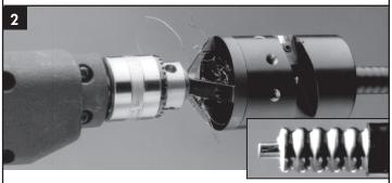
Position the tool on the cable so that it is aligned and start the drill at medium to full speed. Use slight and steady pressure to force the tool along the cable until you feel the detent action as the ball bearings snap into place. The pitch of the motor will also increase. Then, stop the motor, switch to reverse, and withdraw the tool. **Note:** Reversing the motor prevents the cutter blades from striking the outer conductor should the motor accidentaly be restarted.
