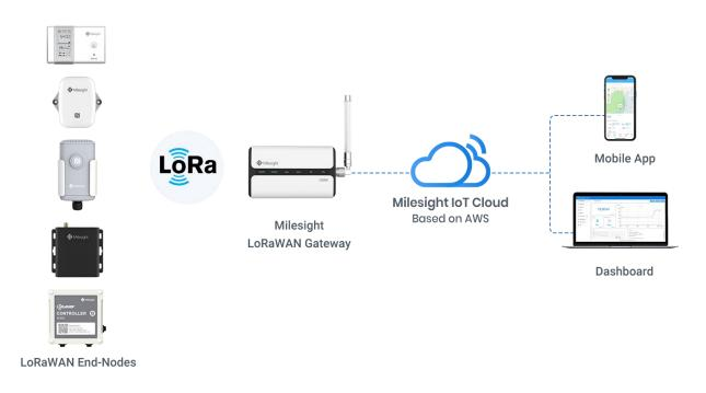
Milesight IoT Cloud provides unparalleled levels of vertical integration with Milesight LoRaWAN® nodes (sensors and controllers). It visualizes field data and enables user to monitor and control remote assets on an intuitive dashboard.
