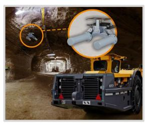
2x HELI-13 antennas mounted on the BRKT-45 for MIMO application
