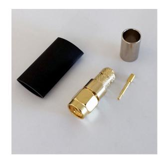
SMA connectors have become the mainstay of wireless technologies thanks to their modest durability and very compact size. The SMA Male (also referred to as an SMA Plug) connector can be identified by its hex-shaped outer body which rotates to interface by its inner thread.
