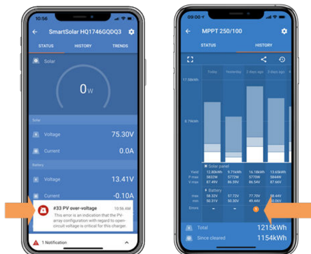
VictronConnect: screenshot of an Error #33 and a screenshot of the history indicating an error
