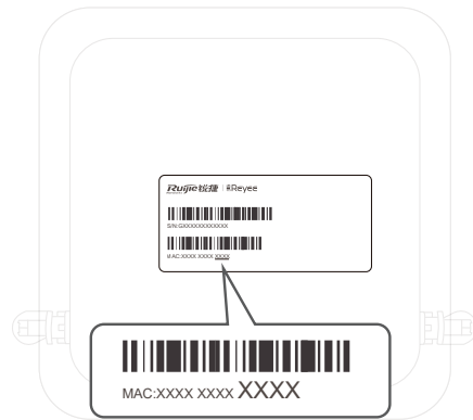
(XXXX refers to the last four digits of MAC on the back of router)
