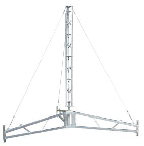
This unique portable lattice tower consists of three sturdy bolt-together aluminium outriggers, a 600 mm aluminium base, a 3.1 metre AL220 lattice section, guy wires, and your choice of 1.0 metre headframe. APAC's AL220 aluminium lattice tower modules feature three upright columns made from 42x3 CHS with 25x3 CHS lattice welded in between by certified boom welders, providing incredible strength while retaining a lightweight design that can support your technician to climb the tripod tower.
