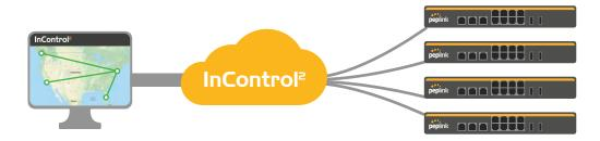
The Balance 310X comes with the InControl central management system. Easily centralize firewall rules, outbound policy, VLAN, device configurations and more.
