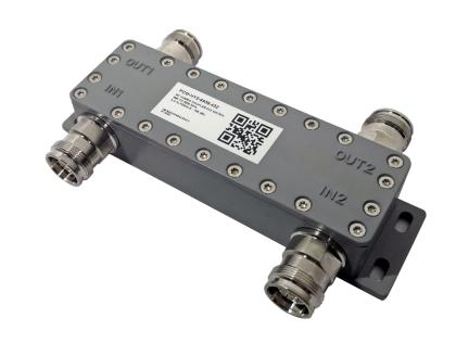
Hybrid Couplers are used to develop advanced RF transmission systems where interaction-free signal combining is required. 2x2 couplers are typically used as an effective means of combining two radio carriers. The unit has two input ports which feed two coupled output ports.
