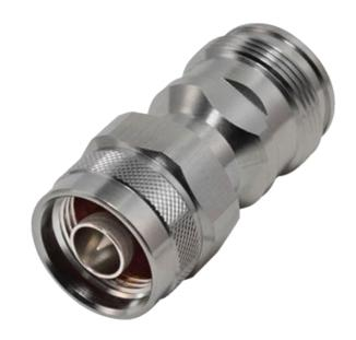
4.3-10 Female to N Male adapters are most commonly used to convert older N-Type antennas to the latest generation 4.3-10 interface. This adapter typically threads onto an N Female interface (such as at the base of an antenna) and allows the attachment of a 4.3-10 feeder cable. This coaxial adapter is IEC 61169-54 and IEC 61169-16 compliant and supports frequencies up to 6 GHz.
