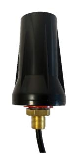
The VST-6927-3 is an economic, high performance stud mount wideband 4G antenna for external use on a range of M2M devices including electronic advertising, vending machines, and metering applications. Stable omnidirectional gain and high efficiency across the entire operating frequency range ensures consistent reception and transmission.
