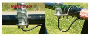
Route the RG58 low loss stranded cable carefully. Avoid high heat areas such as hot components within an engine bay. Ensure that the cable is not stretched excessively and there are no sharp kinks. Use cable ties, but do not pull so tight as to crush the cable. A damaged feeder cable is a cause of high VSWR and reduced performance.
