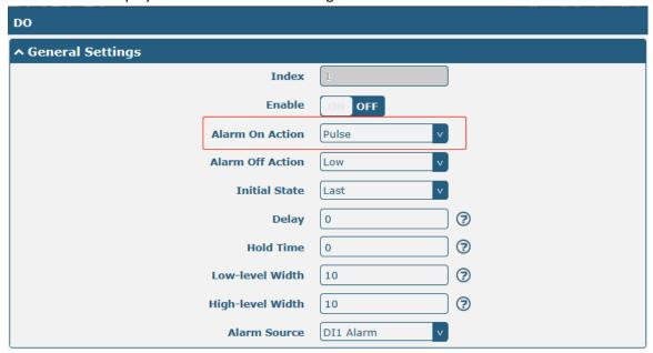
The window is displayed as below when choosing "Pulse" as the alarm off action.
