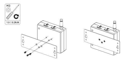
Use 3 pcs of ST2.9\*6 flat head self-tapping Phillips screws to fix the wall mounting kit to the gateway, and then use 2 pcs of M3 drywall screws to mount the gateway associated with the wall mounting kit on the wall.
