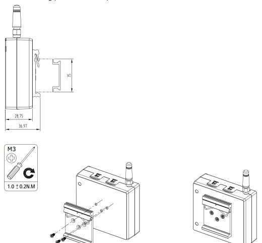
Use 3 pcs of ST3\*8 flat head self-tapping Phillips screws to fix the DIN rail to the gateway, and then hang the DIN rail on the mounting bracket. It is necessary to choose a standard bracket.
