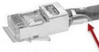
Twisted Braid Enveloped by Crimping Tail
